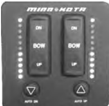
Both Trim Tabs 30° down This is the bottom of Troll Range
